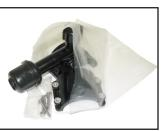
Chamfer end of pipe using <u>Continental's</u> double ended ID chamfering
